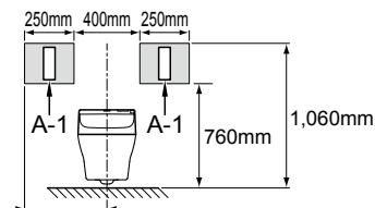
**12** Temporarily place the remote control in the position determined in **11** and confirm the signal reception of A-1.
