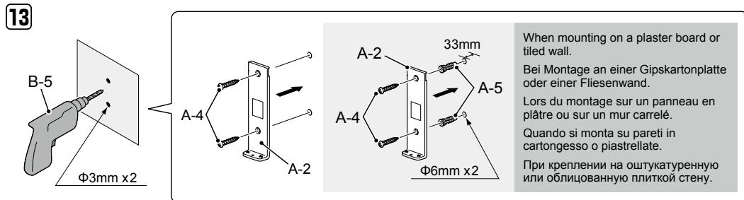
When mounting on a plaster board or tiled wall.
